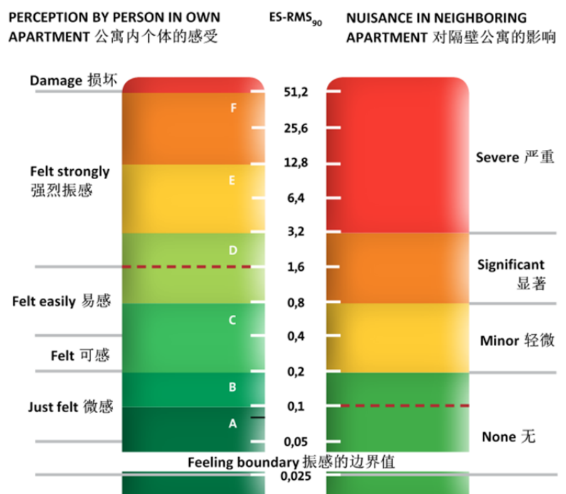
Figure 7. Target values mm/s for vibration level in floor system (Source: Royal HaskoningDHV)
